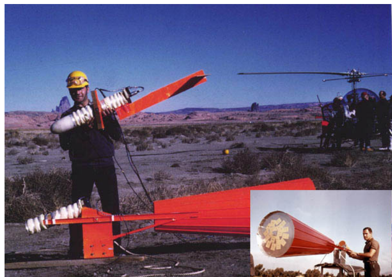
Breiner near Monument Valley, Arizona, testing the first rubidium airborne magnetic gradiometer, October, 1961
