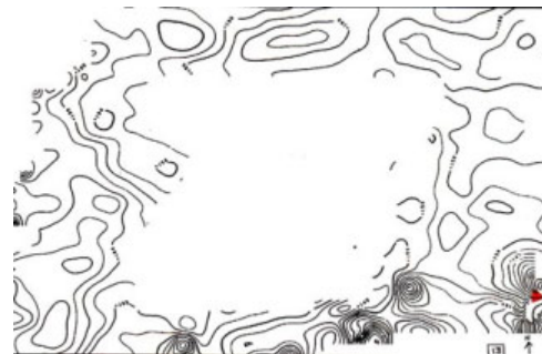
Figure 7. Contour map of magnetic intensity over Monument 61 (shown in Figure 6). The head was found under the anomalous area indicated by the colored marker in the lower right-hand corner of the map. The area at the center of the map was covered by a large artificial pond, where no measurements were made.
