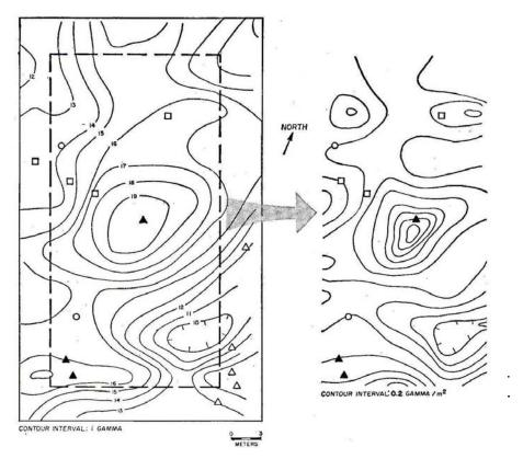
Fig. 9. (Left) Plot (grid 15: Zona Casa Bianca, plain of Sybaris, October 1964) of total magnetic intensity over ruins buried at depths of 3.5 to 6 meters, and results of drilling. (Right) Plot of computed second vertical derivative for the area outlined by dashed lines in the plot at left. (Circles) No results; (squares) drill stopped by wall: (open triangles) resistance from friable material (potsherds); (solid triangles) drill stopped, many potsherds.
