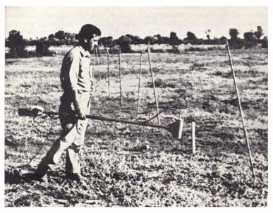
Fig. 6. Beginning a rubidium magnetometer traverse over grid 16 of the exploration site. The area is underlain by a complex of structures at a depth of 3 to 6 meters
