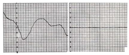
Fig. 3. Rubidium magnetometer recordings from the plain of Sybaris, made with both sensors in a fixed position. Full scale represents 1 gamma; duration of each recording shown, about 7.5 seconds. (Left) Single sensor recording of typical daytime micropulsations. (Right) Differential magnetometer recording made during the same activity, with almost complete cancellation of time variations.
