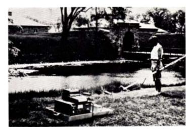
Fig. 2. A differential rubidium magnetometer in use at Fort Lennox, Quebec. The equipment at left makes recordings from the cylindrical sensors on the ground and on the hand-held staff.
