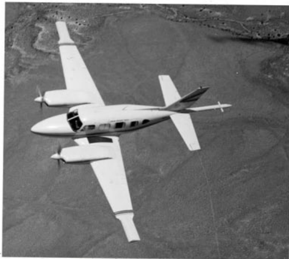
Figure 7: Three-sensor magnetometer installation, one proton magnetometer in each wing tip and one in a tail-mounted stinger. Wing tip sensors constitute a transverse gradiometer. Courtesy, U. S. Geological Survey.
