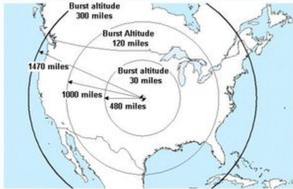
EMP AREA BY BURSTS AT 30, 120 and 300 MILES Gary Smith, "Electromagnetic Pulse Threats", testimony to House National Security Committee on July 16, 1997
